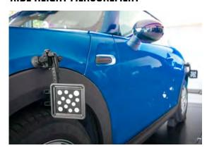
Eliminate manual data entry, speed up measuring, and increase accuracy using our specially designed, optional Ride Height Targets.
